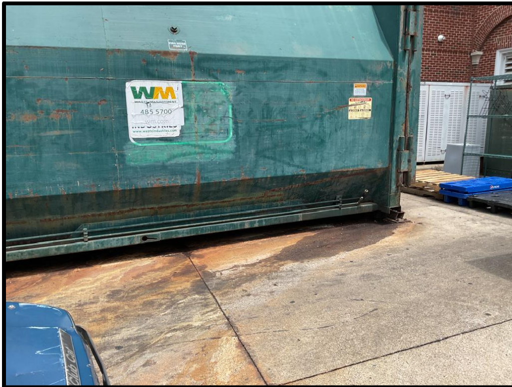
Photo #4: Discharge from trash compactor
